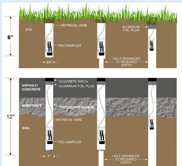
Georgetown. Passive soil gas surveys utilize adsorbent samplers that are placed in the subsurface to adsorb volatile and semivolatile organic compounds (VOCs and SVOCs) in soil gas. Samples are collected by placing a subsurface sampler within an approximately one-inch diameter hole to a typical depth of one to three feet. This method can sample trace levels of compounds in soil gas that result from contamination in soil and/or groundwater. Passive sampling is expected to conclude July 31, 2023.
