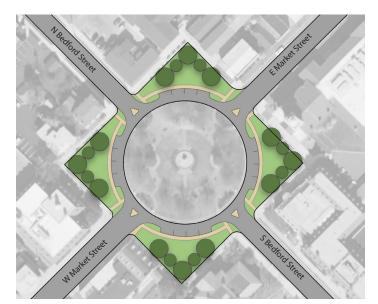
Plan 3 maintains one vehicular lane but adds 16 parallel parking spaces. Parallel parking is safer than back-out parking since motorists exiting these parking spaces will be able to more clearly see on-coming traffic. Also, if accidents occur, all vehicles are moving in the same direction, a condition that usually results in less severe accidents.
