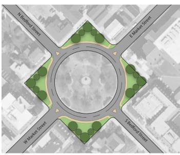
Plan 2 adds a second travel lane with no parking. This may allow smoother vehicle transitions and turns into and out of the circle.
