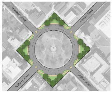
Plan 4 illustrates two lanes of travel with 20 parallel parking spaces. Additional parking is possible since the length of the arc on the outside of the circle is longer.
