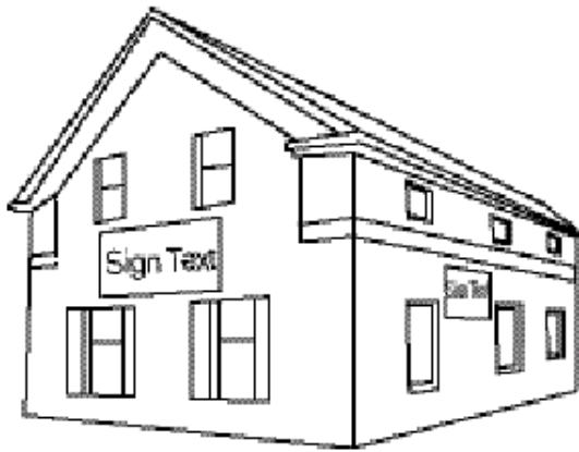
Awkward placement of sign panels.
