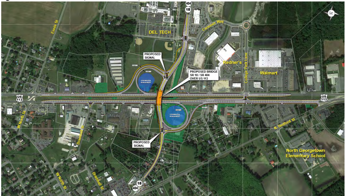
Figure 3-6. US 113 at SR 18/SR 404 Grade Separation
